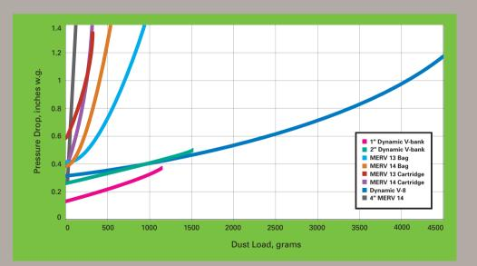
**Unequalled Dust-Loading** Figure 2 The graph at right shows pressure drop as a function of
